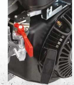
An exclusive to the 5.5-10HP Vanguard<sup>™</sup> engines is the innovative TransportGuard™ system, which requires a simple flip of a switch to turn off the ignition and fuel supply. This prevents fuel flowing into the engine crankcase and diluting the oil during transportation, reducing your customers equipment down time and operating costs, ensuring the equipment arrives on site ready to work, again and again!
